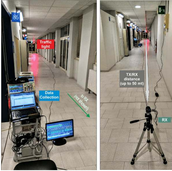
Fig. 4: Experimental campaign: a standard traffic transmits VLC signal to a photo-receiver stage equipped with digital Active Decode and Relay block. The data collection unit consists of a PC and an oscilloscope. The distance between transmitter and receiver is up to 50 m limited by available line of sight length in the building.
